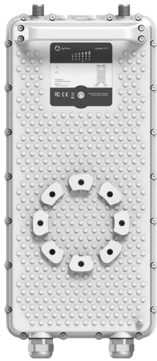
Base-station with N-type connectors for the external antenna
